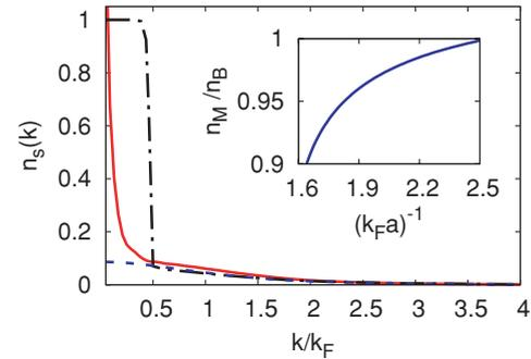
FIG. 4. (Color online) Boson (solid line) and fermion (dash-dotted line) momenta distribution curves for  $n_B = n_F$ ,  $m_B = m_F$ ,  $(k_F a)^{-1} = 1.63$ , and  $T = T_c \simeq 0.015 E_F$ . See text for the meaning of the dashed curve. The inset reports the fraction of molecules vs  $(k_F a)^{-1}$  for the same mixture at  $T = 0.1 E_F$ .
