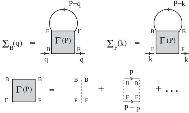
FIG. 1.  $T$ -matrix diagrams for the fermionic and bosonic self-energies in the normal phase. Full lines represent bare bosonic (BB) and fermionic (FF) Green's functions. Broken lines represent bare boson-fermion interactions  $v_0$ .
