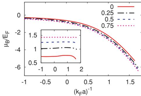
FIG. 3. (Color online) Boson chemical potential at the critical temperature  $T_c$  (in units of  $E_F$ ) vs the boson-fermion coupling  $(k_F a)^{-1}$  for different values of the density imbalance  $(n_F - n_B)/n$  in a mixture with  $m_B = m_F$ . The corresponding fermion chemical potential is reported in the inset.
